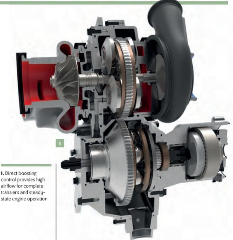
Direct boosting control provides high airflow for complete transient and steady-
